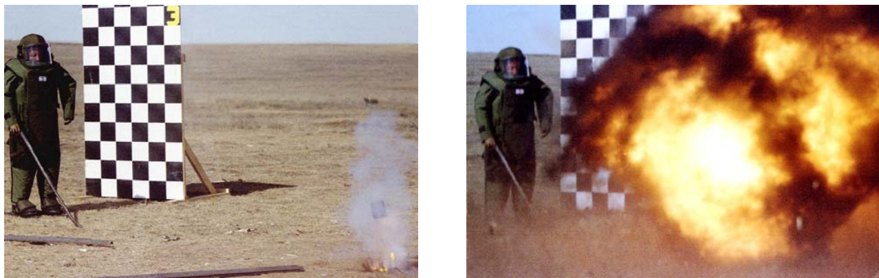
Figure 2: Explosion of a Bounding Fragmentation Mine in front of a Mannequin Wearing PPE. (Pictures Courtesy of DRDC, Canada)
